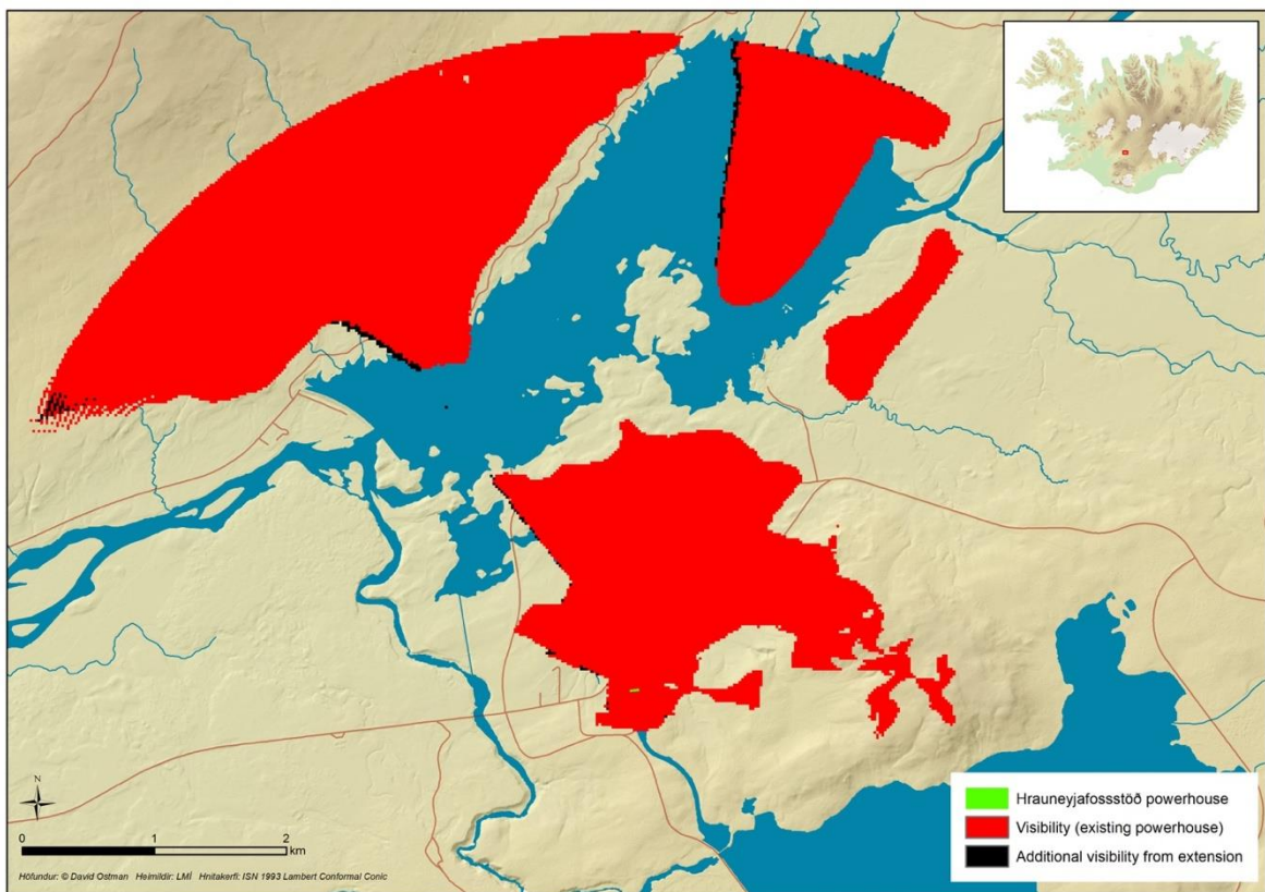
Fig. 13. Visibility results before (RED) and after (BLACK) the planned powerhouse extension for Hrauneyjafosstöð
