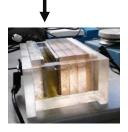
$\begin{array}{l} \text{Plexiglass,} \\ \text{20} \times \text{8} \times \text{2.5 cm} \end{array}$
